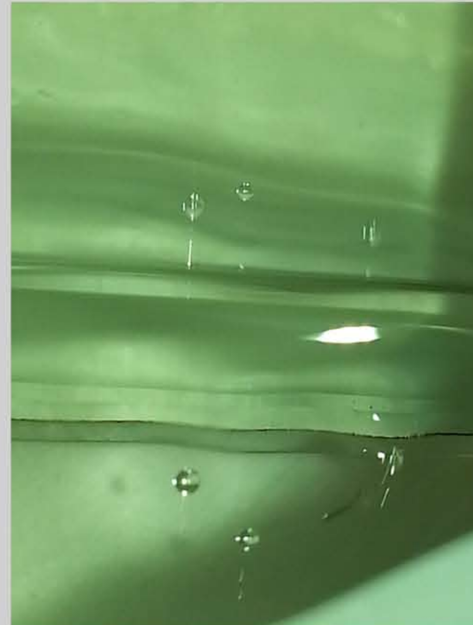
Three jumping droplets on silicon oil. To better determine the height of the jumps, a mirror was placed behind the droplets. (50 cSt, U=2.98 V, I=0.54 A)
